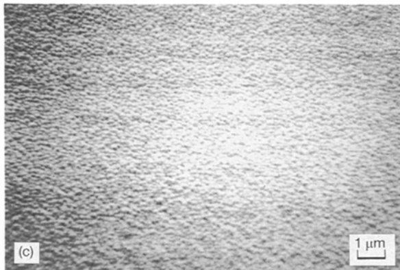
Figure 4 Effect of percentage change in argon pressure on the microstructure of \text{Bi}_4\text{Ti}_3\text{O}_{12} thin films. (a) 10 mtorr, (b) 15 mtorr, (c) 20 mtorr.
